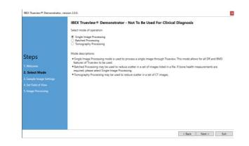
If the user wishes to interactively select images and select the appropriate inputs (kV, Filters, etc.) the default mode '**Single Image Processing**' should be selected. Examples of interactive operation for 'DR' and 'Bone health' modalities have been recorded on pages 4 and 5. The workflow for the 'Mammography' modality is the same as for 'DR'. The full set of services are available to the user in this mode.
