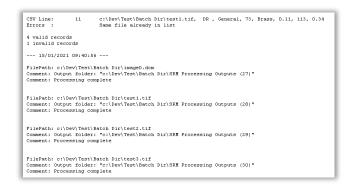
When the CSV file is loaded, the GUI reports the number of records that can be processed, and any records that have problems. Any problems are reported in the log file. The example here indicates that the same image has been listed more than once.
