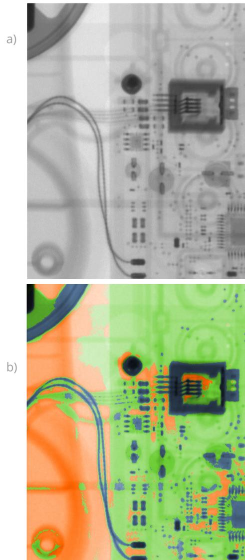
Figure 3: Close-up of a region of Figure 2. a): MAP-stripped absorption contrast image. b): materials classified overlay image.
