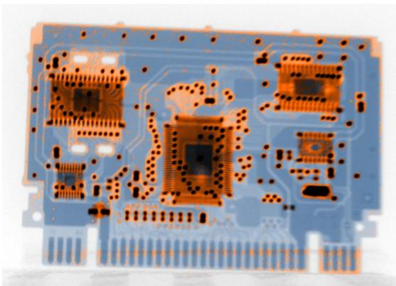
Figure 1: Materials classified image of a PCB, collected using a portable, pulsed X-ray generator running at 100 kVp, 1 mA and a flat panel detector with 127  $\mu\text{m}$  pixel size. Regions of the image classified as organic material are coloured orange, and metals, blue. There are no "poor" metals (normally coloured green). Classification limits applied, leaving some regions of the image
