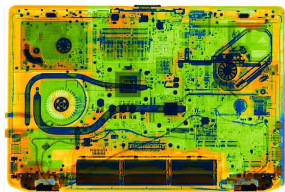
Figure 4: Materials classified image of a laptop, collected using a portable, continuous X-ray generator running at 120 kVp and a line-scanner detector. Classification limits not applied.
