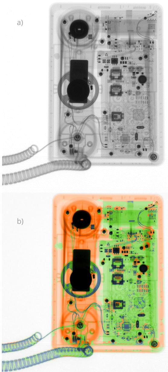
Figure 2: a): MAP-stripped absorption contrast image of a telephone. b): materials classified image. Continuous X-ray generator running at 120 kVp, flat-panel detector with 127  $\mu\text{m}$  pixel size. Classification limits applied.
