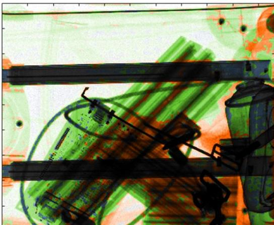
*Figure 5: Materials classified image of objects in a carry-on suitcase, collected using a portable, continuous X-ray generator running at 120 kVp and a line-scanner detector. Classification limits applied. It is not unusual in a security scanning system for heavier plastics such as PVC to be classified as poor metals but judicious choice of training materials, or a bias in the analysis, can get around this.*
