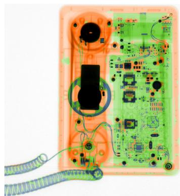
Figure 7: An IBEX classified image of a telephone. Plastics appear orange, lighter metals appear green, and denser metals blue. Where the X-ray beam passes through multiple materials, the classification reflects the average material type.
