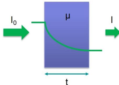
Figure 1: Illustration of the Beer-Lambert Law, describing the absorption of X-rays by a material.
