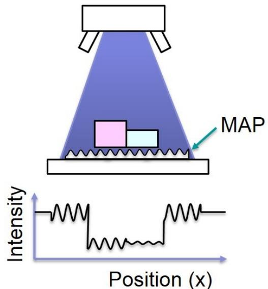
Figure 3: The IBEX MAP introduces modulations into the X-ray absorption image, enabling energy-dependent information to be obtained which gives access to material information.
