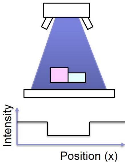
Figure 2: Thicker, less dense material can look the same as thin, dense material in a conventional X-ray system.
