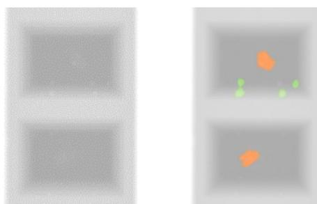
Figure 8: A MAP-stripped absorption contrast image (left) of chocolate chunks deliberately contaminated with plastic fragments. The contaminants are difficult to see. Right: IBEX technology identifies departures from “normal” product and distinguishes between unusual bubbles (green) and contaminants (orange).
