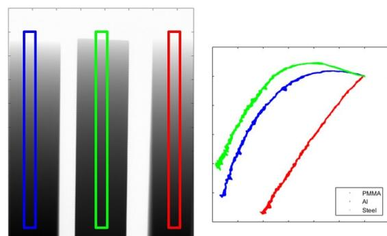
Figure 4: Left: regions of interest covering the thickness ranges of training wedges of (from left to right) aluminium, steel and PMMA. Right: the materials signatures traced in IBEX materials space, showing the materials clearly distinguished.
