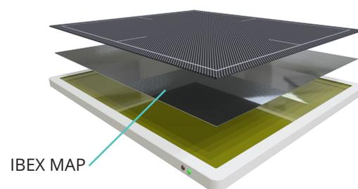
Figure 1: Standard DR configuration, with the addition of the IBEX MAP.
