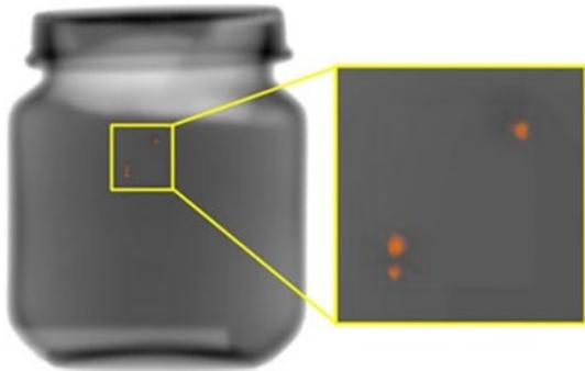
Figure 3: IBEX materials technology detects the contaminants. Here, they are highlighted in orange overlaid on the MAP-stripped absorption contrast image.
