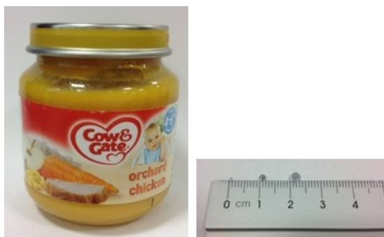
Figure 1: Left: one of the jars of puréed baby food used in the trial. Right: glass beads deliberately introduced as contaminants.
