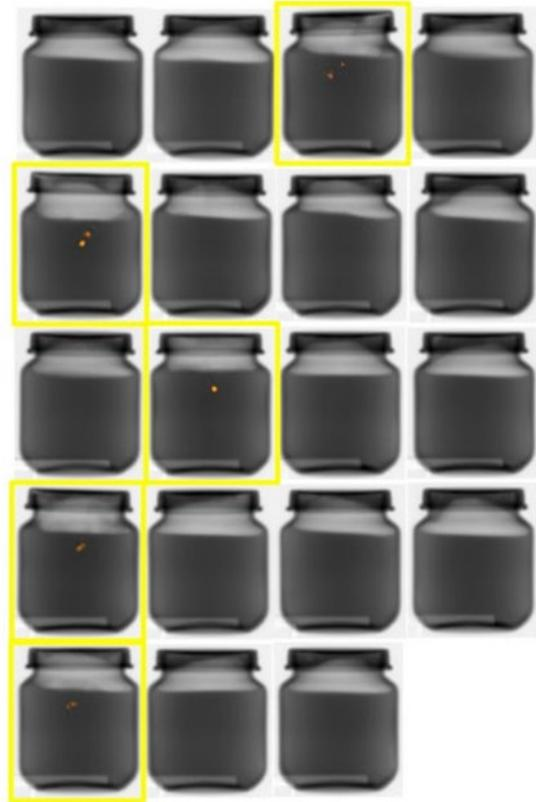
Figure 4: MAP-stripped absorption contrast images of all 19 jars in the test set. The glass contaminants were successfully detected in the five contaminated jars. These are framed in yellow with the contaminants themselves highlighted in orange.
