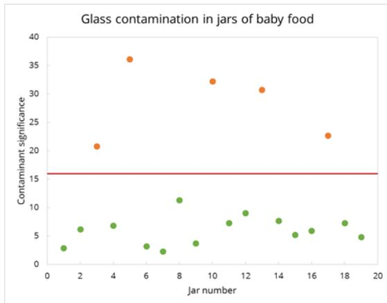
Figure 5: Quantitative measures of “contaminant significance” enable thresholding in a production QA environment. This test showed clear differences in this measure between contaminated and non-contaminated samples.
