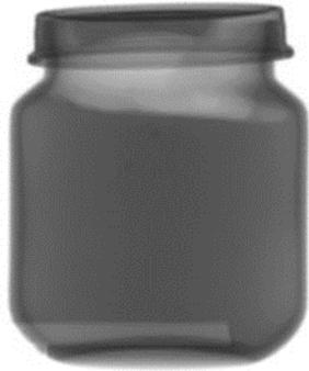
Figure 2: Absorption contrast image of a contaminated jar of baby food. The glass bead contaminants are barely visible. The pale rectangle in the bottom left of the image comes from the alignment jig used in this test where the samples were positioned manually.
