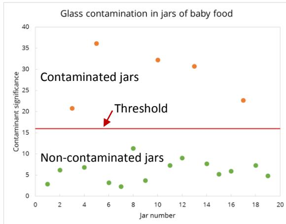
Figure 7: Quantitative measures of “contaminant significance” enable thresholding in a production QA environment. This test showed clear differences in this measure between contaminated and non-contaminated samples.
