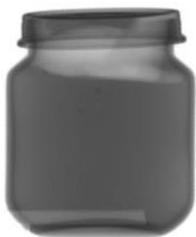
Figure 4: Absorption contrast image of a contaminated jar of baby food. The glass bead contaminants are barely visible. The pale rectangle in the bottom left of the image comes from the alignment jig used in this test where the samples were positioned manually.
