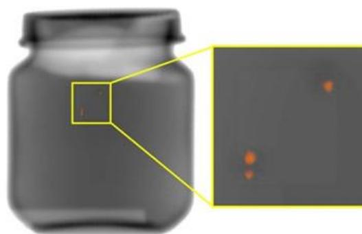
Figure 5: IBEX materials technology detects the contaminants. In the image above, they are shown in orange.
