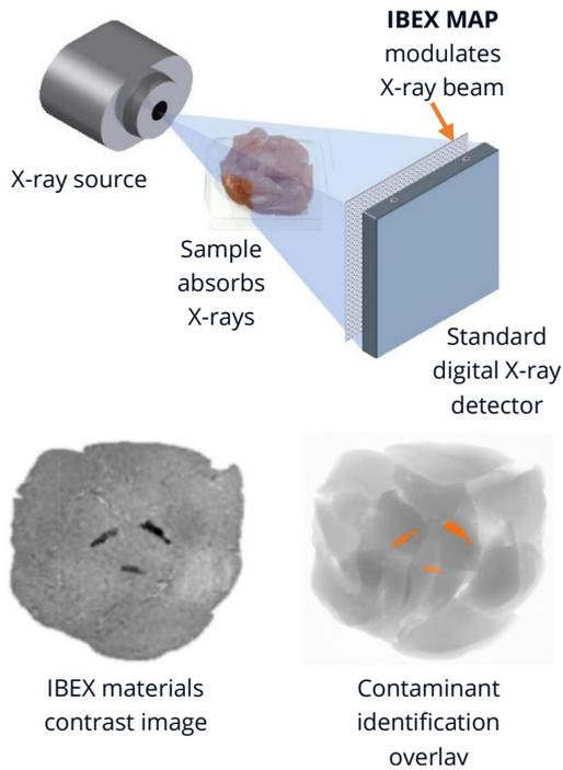
Figure 2: An IBEX MAP-enabled system. The MAP modulates the image in a predictable manner, allowing recovery of energy-dependent information leading to construction of a materials contrast image, as seen above.
