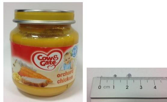
Figure 3: Left: one of the jars of puréed baby food used in the trial. Right: glass beads used for the contamination.
