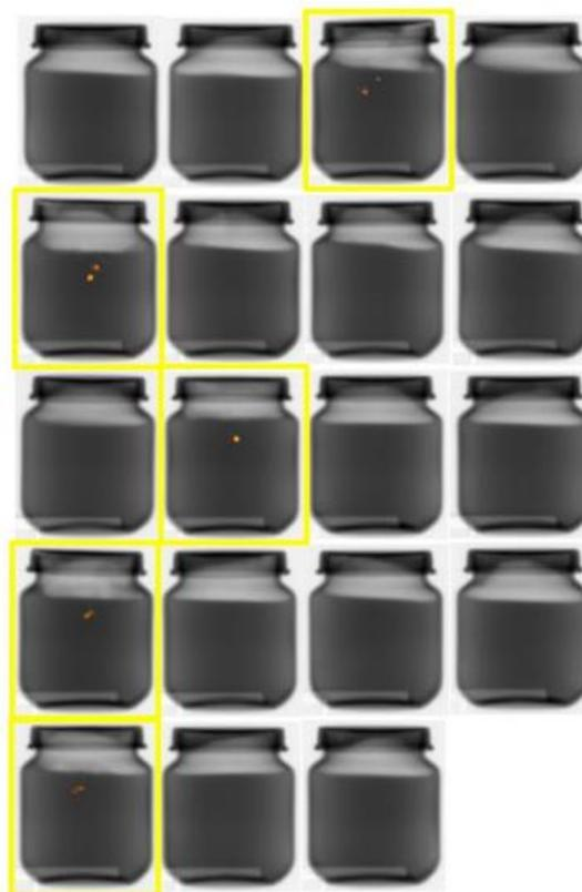
Figure 6: Absorption contrast images of all 19 jars in the test set. The glass contaminants were successfully detected in the five contaminated jars. These are framed in yellow, with the contaminants themselves highlighted in orange.
