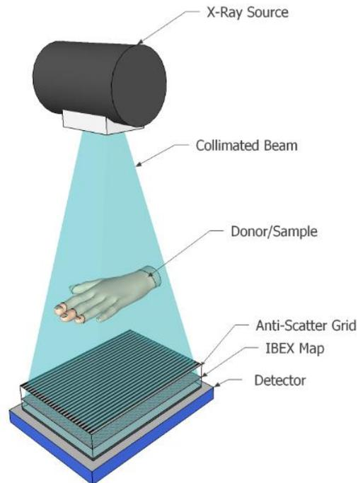
Figure 1: Standard DR configuration, with the addition of the IBEX MAP, for measurements on cadaver donor parts. Not to scale.
