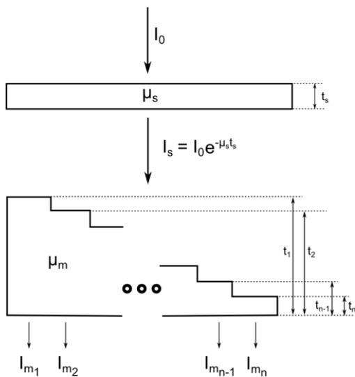
Figure 2: Impact of an IBEX MAP structure on an incident monochromatic X-ray beam.
