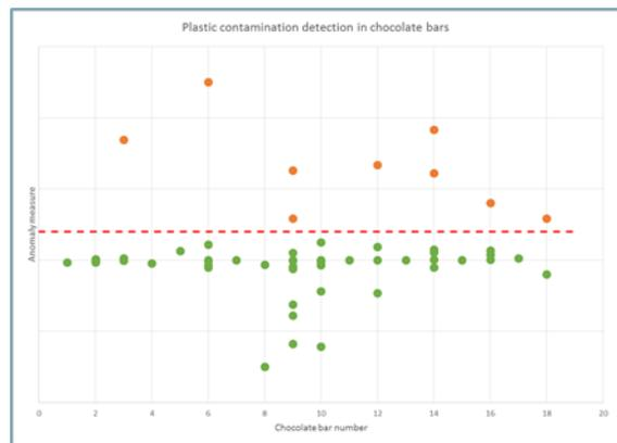
Figure 4: Quantitative scoring of the degree of anomaly compared to normal chocolate. Above the threshold (red dashed line), the anomaly measure indicates plastic contamination. Below the threshold is normal or deformed chocolate.
