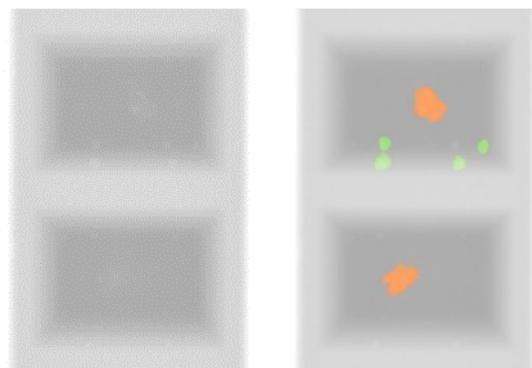
Figure 1: Left: X-ray absorption contrast image of Bar 14. Right: IBEX materials classification overlay image. Plastic contaminated regions are highlighted in orange; unusual bubbles or deformed areas of chocolate are highlighted in green.
