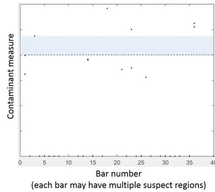
Figure 6: A plot of anomaly (or contaminant) measure, with a threshold set (dotted line). There is a clear distance (pale blue panel) between wafer bars containing contaminants (above) and clean bars (below the threshold).
