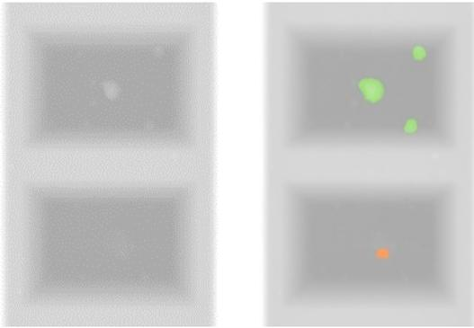
Figure 2: Bar 16. Left: absorption contrast image, obtained by stripping out the shadow of the MAP from the data. Right: IBEX materials classification overlay: deformed chocolate and bubbles are highlighted in green; contaminated regions in orange. The region identified as containing plastic is barely detectable in the absorption contrast image.
