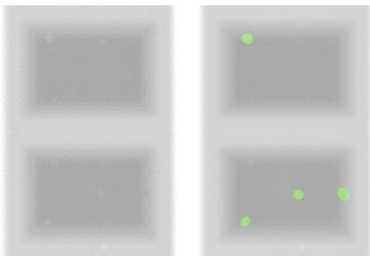
Figure 3: Bar 2. A few bubbles are apparently visible in the X-ray absorption contrast image (left). These are not all highlighted in the materials image (right) since some of them are regular features in the clean bars used to train the model of a normal bar. The unusual bubbles are highlighted and correctly identified as being deformed chocolate and not plastic contamination (right).
