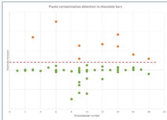
Figure 6: Quantitative scoring of the degree of anomaly compared to normal chocolate. Above the threshold (red dashed line), the anomaly measure indicates plastic contamination. Below the threshold is normal or deformed chocolate.
