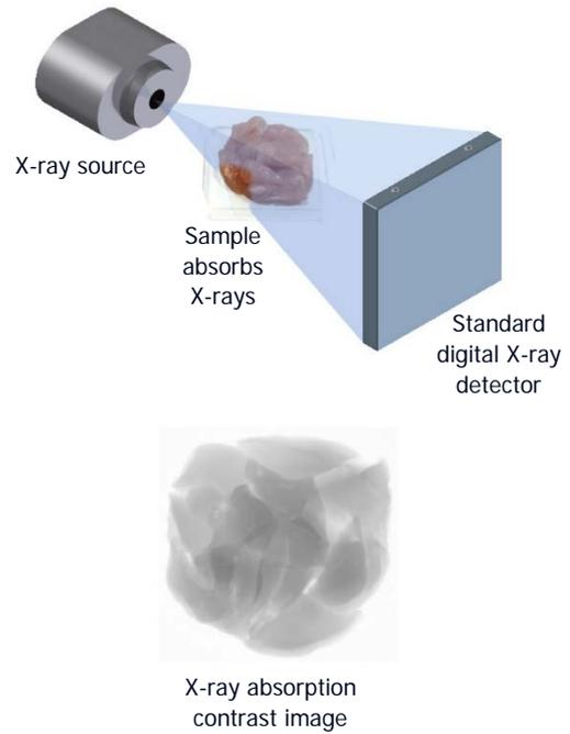
Figure 1: Conventional X-ray absorption contrast imaging. The X-ray source delivers a spectrum of energies. The X-rays are attenuated by the sample according to the materials and their thicknesses in the path of the beam, resulting in an absorption contrast image.
