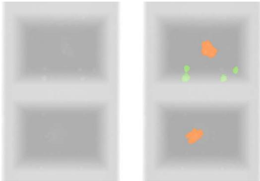
Figure 3: Left: X-ray absorption contrast image of Bar 14. Right: IBEX materials classification overlay image. Plastic contaminated regions are highlighted in orange; unusual bubbles or deformed areas of chocolate are highlighted in green.
