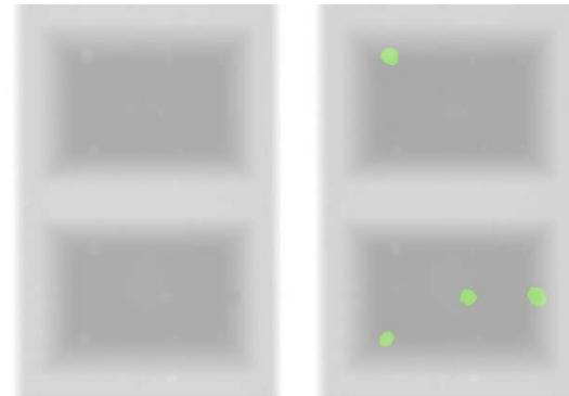
Figure 5: Bar 2. A few bubbles are apparently visible in the X-ray absorption contrast image (left). These are not all highlighted in the materials image (right) since some of them are regular features in the clean bars used to train the model of a normal bar. The unusual bubbles are highlighted and correctly identified as being deformed chocolate and not plastic contamination (right).
