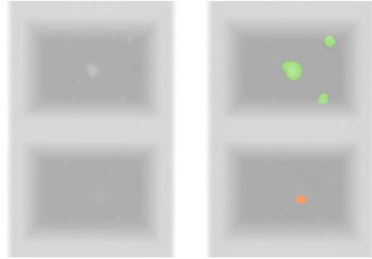
Figure 4: Bar 16. Left: absorption contrast image; right: IBEX materials classification overlay: deformed chocolate and bubbles highlighted green, plastic contaminated region highlighted in orange. The region identified as containing plastic is barely detectable in the absorption contrast image.
