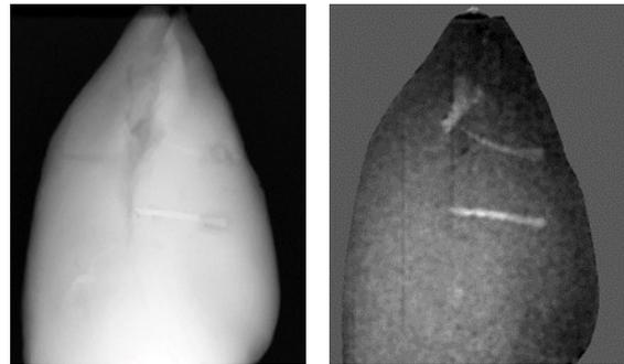
Figure 6: Absorption contrast image (left) of the chicken breast sample containing three bone fragments deliberately placed. Right: IBEX materials contrast image, revealing the locations of all three bone fragments (light contrast). From top to bottom: fan bone, rib, rib.
