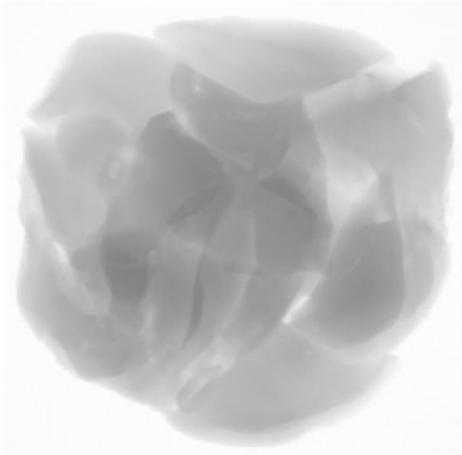
Figure 4: Absorption contrast image of the diced chicken sample, with the effect of the IBEX MAP stripped out. The locations of the bone fragments are not evident from this image, as there are different grey-levels in different areas, and shapes and edges do not give reliable clues.
