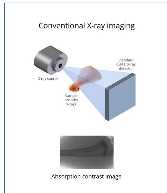
Figure 1: Traditional X-ray absorption contrast imaging. The X-ray source delivers a spectrum of energies. The X-rays are attenuated by the sample according to the materials and their thicknesses in the path of the beam.
