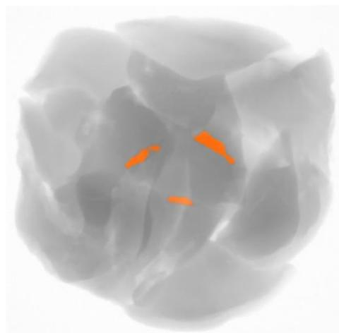
Figure 7: The positions of the bone fragments overlaid on the absorption image of the contaminated diced chicken sample.
