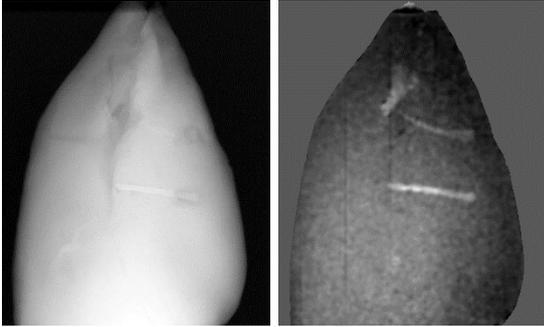
*Figure 8: Absorption contrast image (left) of a whole large chicken breast containing three bone fragments. The bones are hard to see, although the eye picks out one of the ribs quite readily. Right: IBEX materials contrast image, revealing the locations of all three bone fragments (light contrast). From top to bottom: Fan bone, rib, rib.*
