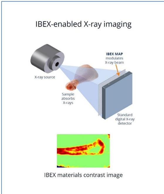
Figure 2: An IBEX MAP-enabled system. The MAP modulates the image in a predictable manner, allowing reconstruction of a materials image.
