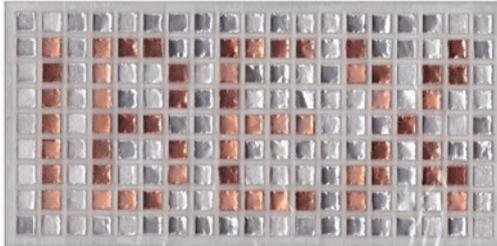
*Test mosaic made of copper and silver tiles of different thicknesses, in a plastic grid.*
